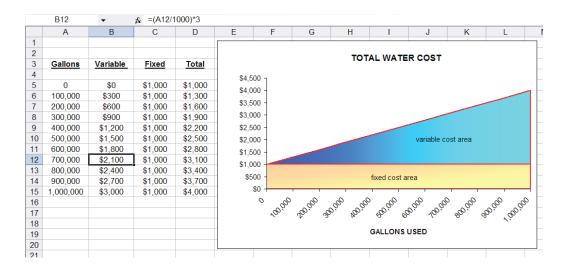
Look closely at the data in the spreadsheet, and notice that the "variable" portion of the water cost is \$3 per thousand gallons. For example, spreadsheet cell B12 is \$2,100 (700 thousand gallons at \$3 per thousand); observe the formula for cell B12 in the upper bar of the spreadsheet (=(A12/1000)\*3). In addition, the "fixed" cost is \$1,000, regardless of the gallons used. The total in column D is the summation of columns B and C. The cost components are mapped in the diagram at the right.
