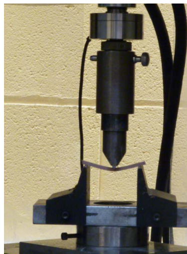
Figure 6.14 A specimen tested in 3-point bending
