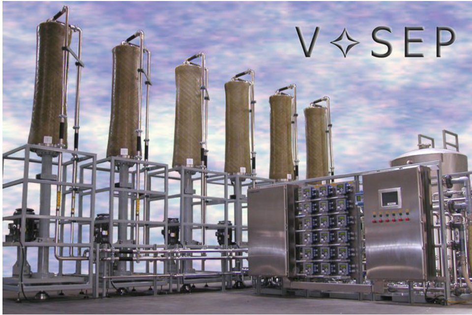
Fig 23. Industrial VSEP modules with 150 m² of membranes
