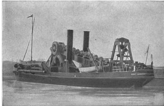
Fig. 8.—Twin-screw hopper-dredger, "Percy Sanderson," built for the European Danube Commission by Wm. Simons & Co.
