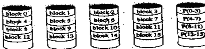
(e) RAID 4 (Block Level Parity of data bits)
