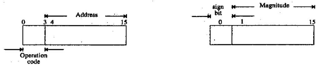
Figure 10: Instruction and data format for an assumed machine
