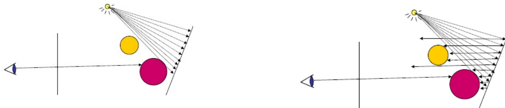
(A) Light leaves the light source, (B) Light leaves the light source, is reflected off the back wall
