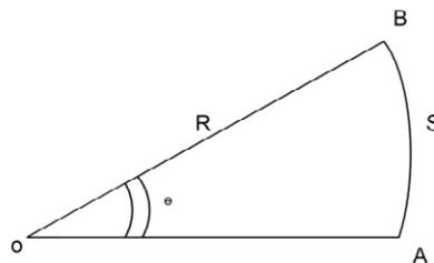
other end A moves from A to B along a circular arc of length S. The angle  $\vartheta$  which measures the inclination between OA and OB is defined by
