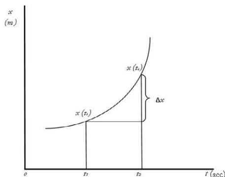
**Average Velocity Vector:** Measures rate of change of position with time over a finite time interval  $(t_2 - t_1)$
