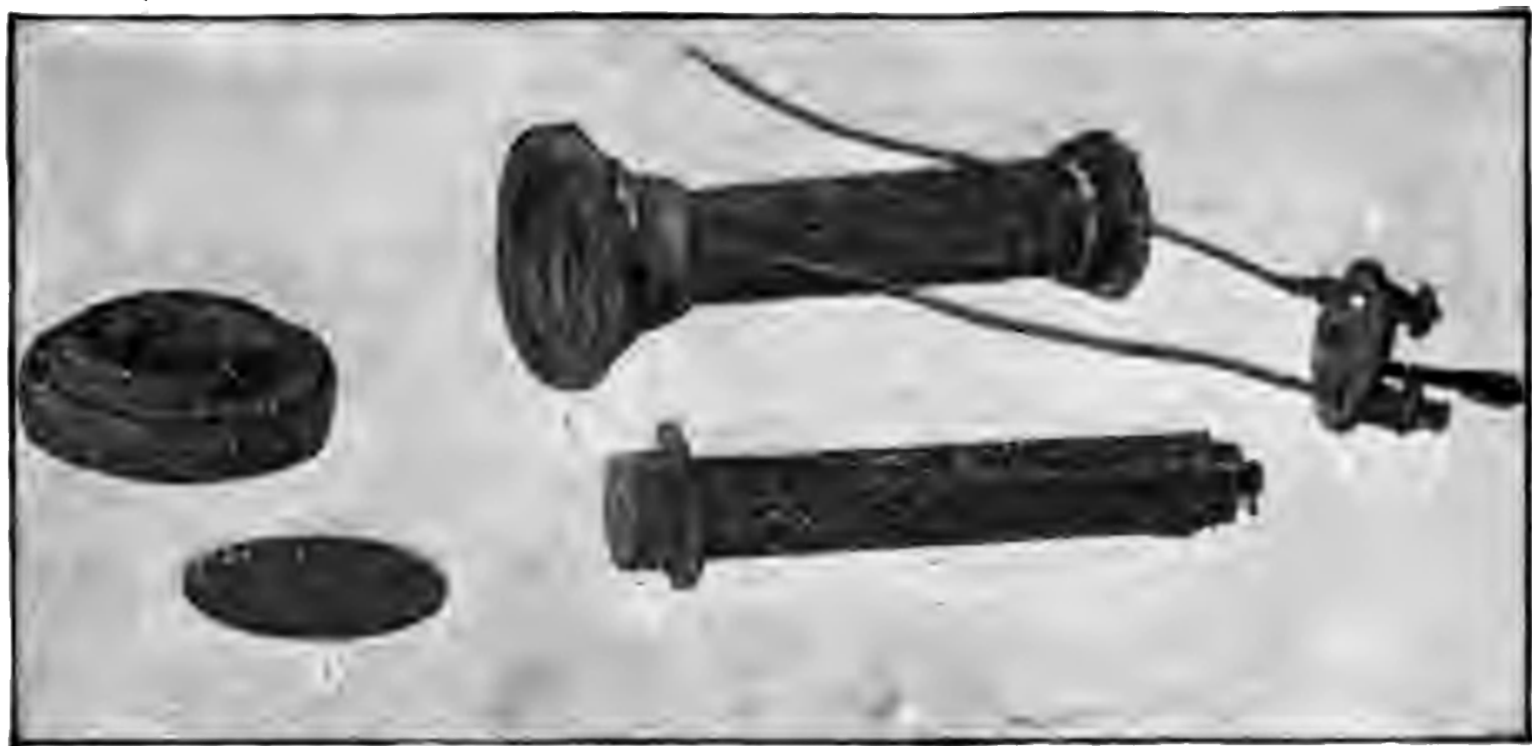
FIG. 56.—PARTS OF AN ORDINARY BELL TELEPHONE.
