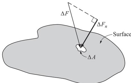
**Figure 1.7** The normal component of a force.
