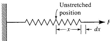
**Figure 3.7** Work needed to stretch a spring.
