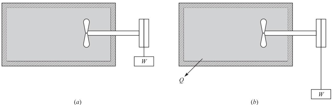
**Figure 4.1** The first law applied to a cycle.
