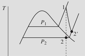
Note that the irreversibility has the desired effect of moving state 2 into the superheated region, thereby eliminating the formation of droplets due to the condensation of moisture. In an actual turbine, moisture formation cannot be tolerated because of damage to the turbine blades, so the irreversibility is somewhat desirable.
