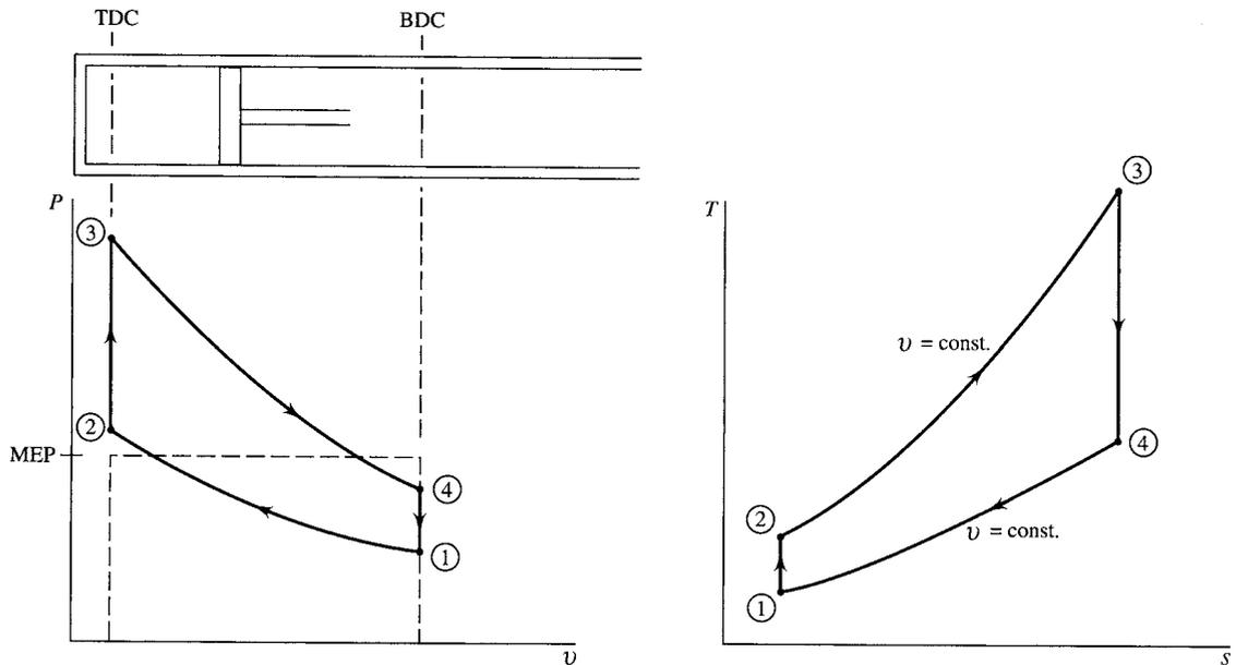
**Figure 7.1** The cycle of a piston-cylinder gasoline engine.
