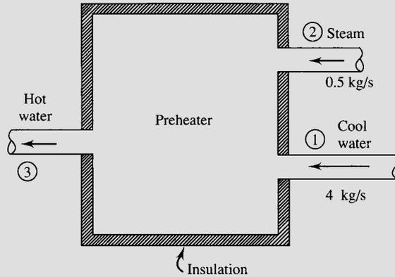
The first law allows us to calculate the temperature of the exiting water. Neglecting kinetic energy and potential energy changes and assuming zero heat transfer, the first law takes the form  $\dot{m}_3 h_3 = \dot{m}_2 h_2 + \dot{m}_1 h_1$ . Using the steam tables ( $h_1$  is the enthalpy of saturated liquid at  $45^\circ\text{C}$ ),
