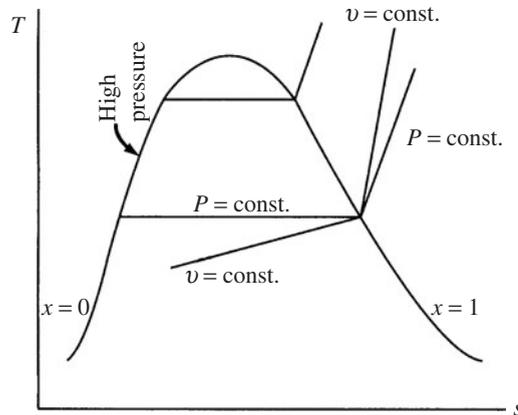
**Figure 5.8** The  $T$ - $s$  diagram for steam.
