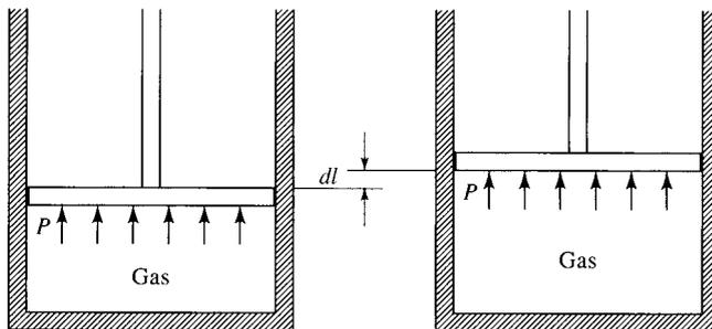
**Figure 3.3** Work due to a moving boundary.
