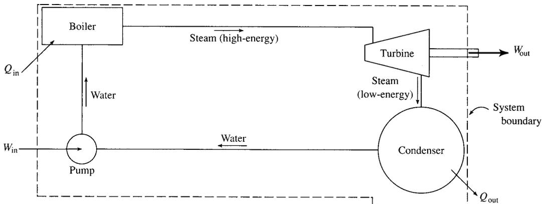
Figure 4.3 A schematic for a power plant.
