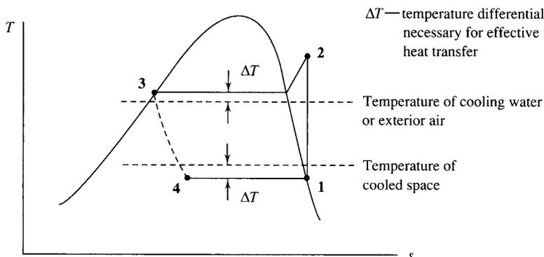
**Figure 6.11** The refrigeration cycle showing design temperatures.
