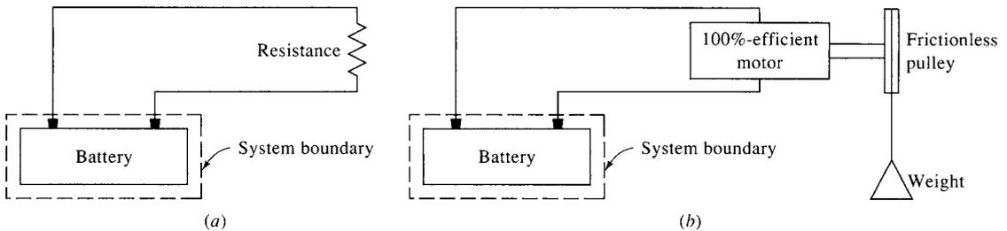
**Figure 3.2** Work being done by electrical means.
