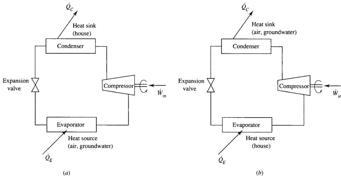
**Figure 6.12** The heat pump. (a) Heating. (b) Cooling.
