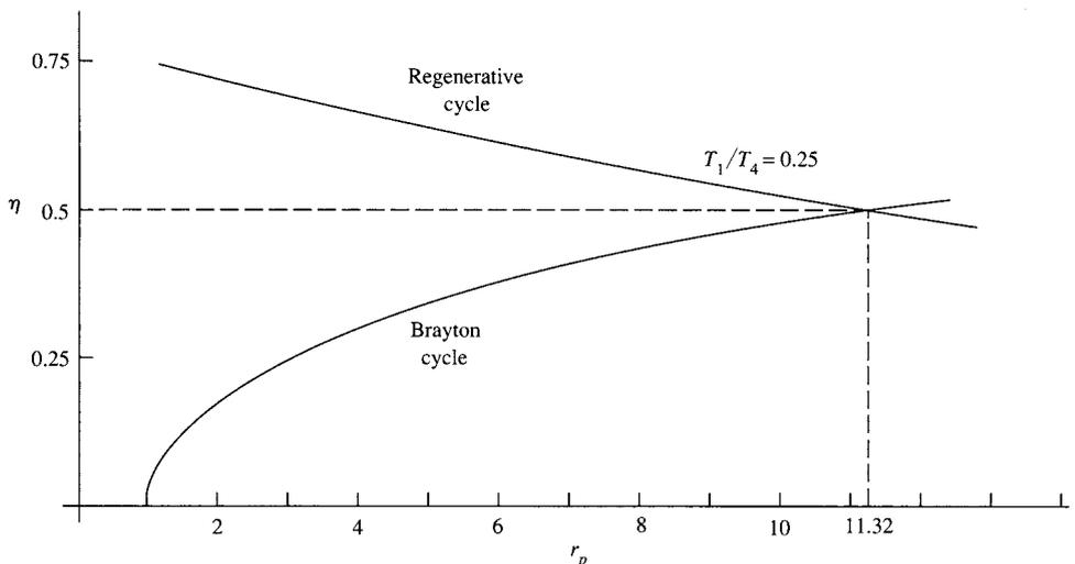
**Figure 7.7** Efficiencies of the Brayton and regenerative cycles.
