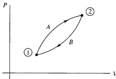
**Figure 4.2** A cycle composed of two processes.
