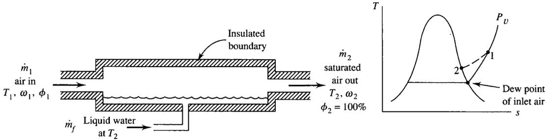
**Figure 8.2** Setup used to find  $\omega$  of air.
