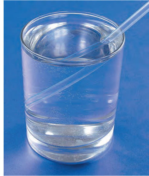
figure 17.10 When viewed from above, a straw appears to bend when part of it is above water and the rest below. Viewed from the side, the straw is magnified.
