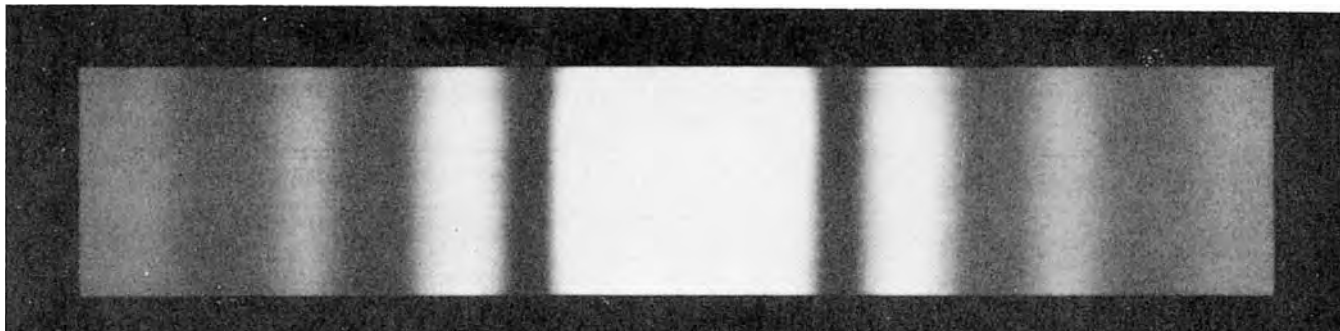
figure 16.17 The diffraction pattern for a narrow single slit has a series of light and dark fringes on either side of a bright central fringe.
