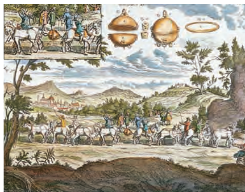
figure 9.8 Two teams of eight horses were unable to separate von Guericke's evacuated metal sphere. What force pushes the two hemispheres together?
