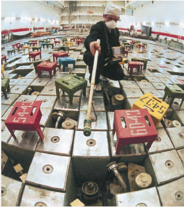
The top of a Chernobyl-type reactor, showing a technician working on the square tops of the fuel-rod assemblies.
