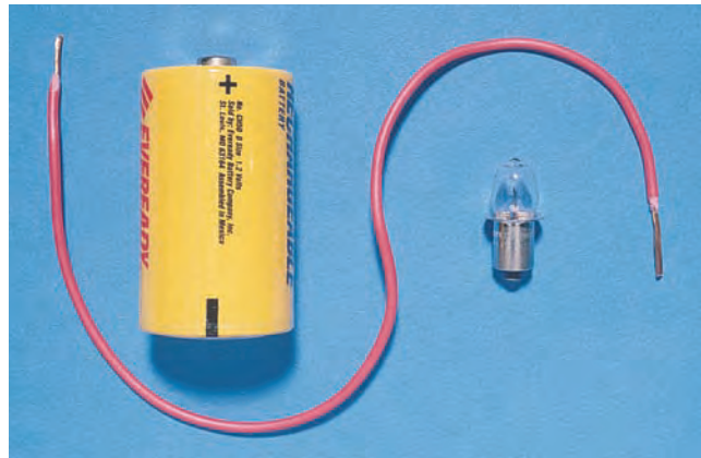
figure 13.1 A battery, a wire, and a flashlight bulb. Can you get the bulb to light?
