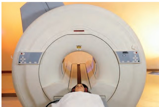
figure 21.19 A patient is about to enter the chamber housing the superconducting magnets of a magnetic resonance imaging (MRI) instrument.
