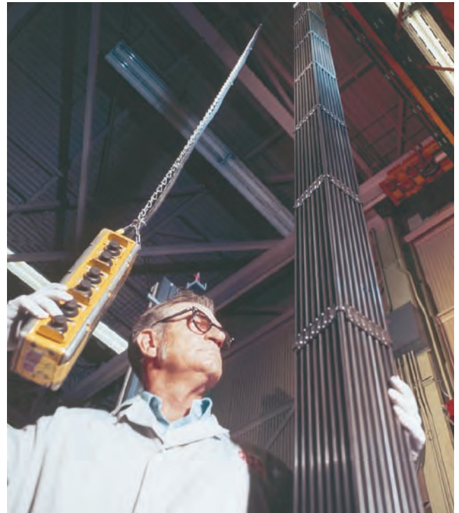
figure 19.17 An assembly containing fuel elements and control rods for use in a modern power reactor.
