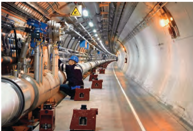
figure 1.7 A Super-Proton-Synchrotron (SPS) particle accelerator used to study interactions of subatomic particles at high energies. It is located at CERN, the European particle-physics laboratory in Switzerland.
