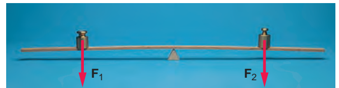
figure 8.5 A simple balance with equal weights placed at equal distances from the fulcrum.
