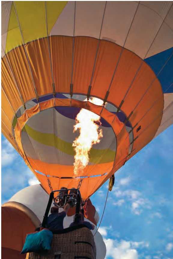
figure 10.17 Heat is added to the air in a hot-air balloon by the propane burner above the gondola. The heated air expands making it less dense than the surrounding air.
