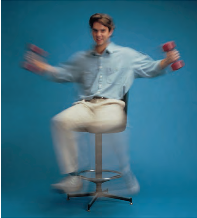
figure 8.17 A student holding masses in each hand while sitting on a rotating stool can achieve a large increase in rotational velocity by bringing his arms in toward his body.
