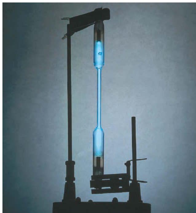
figure 18.16 A high voltage placed across the electrodes of a gas-discharge tube produces a colorful glow. The colors are characteristic of the type of gas in the tube.
