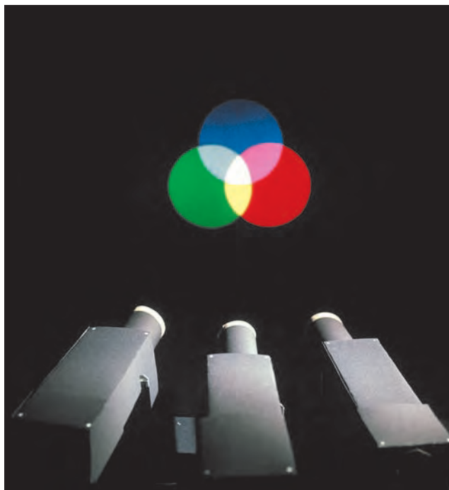
figure 16.9 Additive color mixing is demonstrated by projecting blue, green, and red light from separate projectors onto overlapping circles on a screen.
