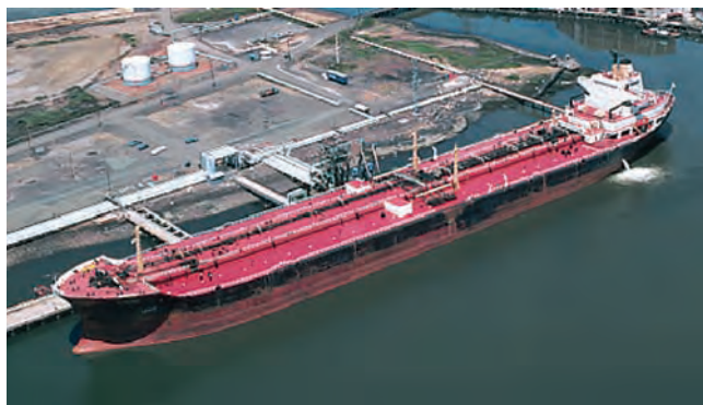
figure 9.16 A fully loaded tanker rides much lower in the water than an empty tanker.
