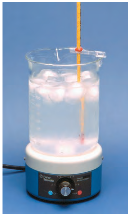
figure 10.10 Adding heat to a mixture of water and ice at 0^\circ\text{C} melts the ice without changing the temperature of the mixture.
