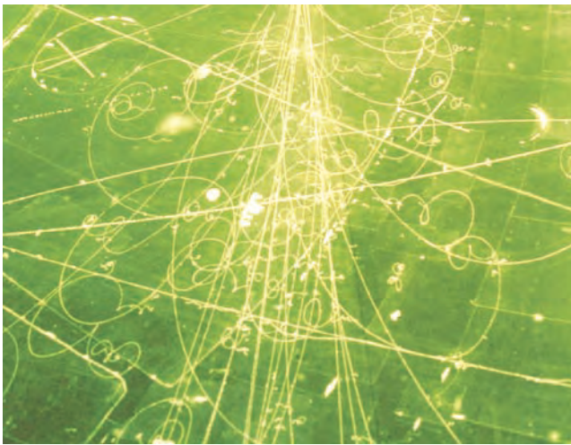
figure 21.3 Particle tracks in a bubble chamber provide information on the new particles produced in collisions or decays.
