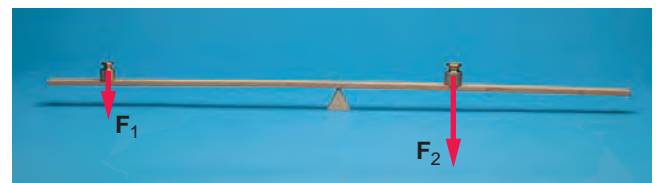
figure 8.6 A simple balance with unequal weights placed at different distances from the fulcrum. What determines whether the system will be balanced?
