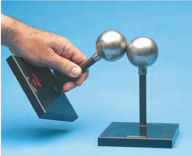
figure 12.12 By bringing two identical metal balls into contact, one charged and the other one initially uncharged, equal quantities of charge are obtained on the two balls.
