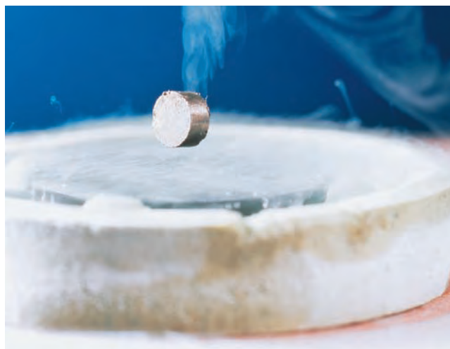
figure 21.17 A small magnet levitates above a superconducting disk cooled with liquid nitrogen. This simple test establishes the presence of superconductivity.
