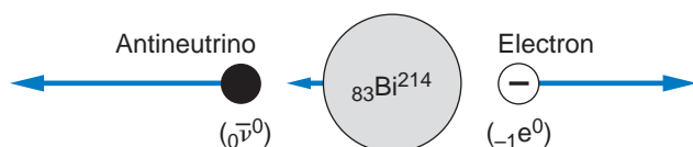
figure 19.7 Beta decay of lead-214. The daughter isotope, bismuth-214, has a higher atomic number than lead.
