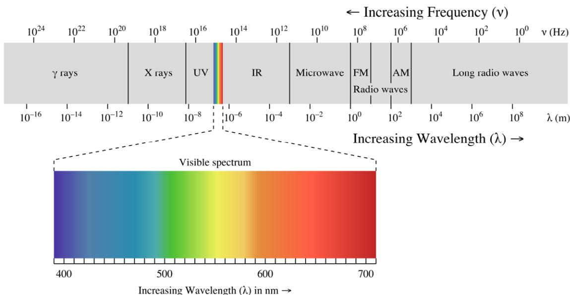
**Figure 2:** Electromagnetic radiation spectrum (courtesy of [Wikipedia.org](https://en.wikipedia.org))
